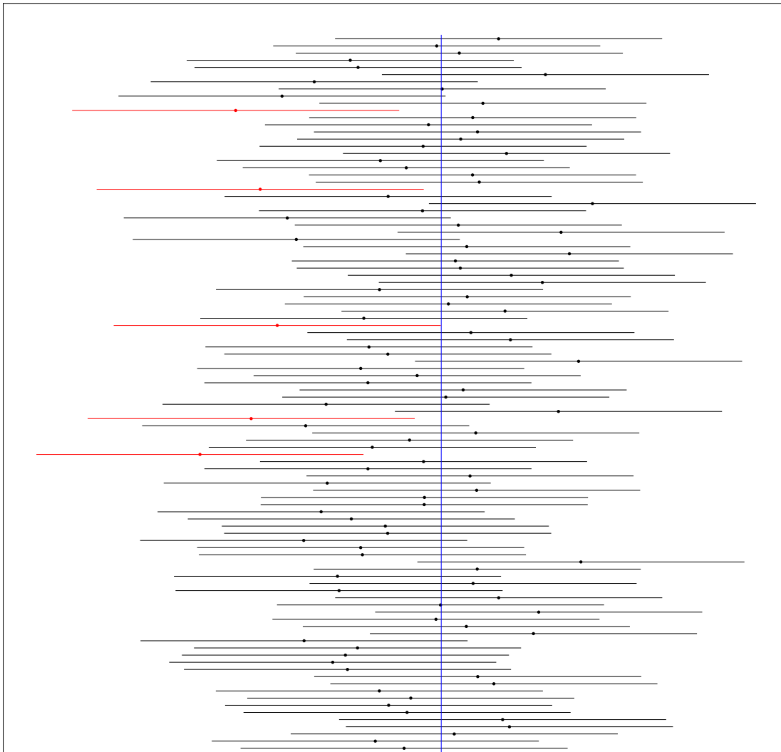
Figure 18.6. Here are one hundred 95% confidence intervals for the mean from a Monte Carlo simulation of a sample of size 5 independent standard normals. The intervals that do not include the true mean 0 are shown in red.
